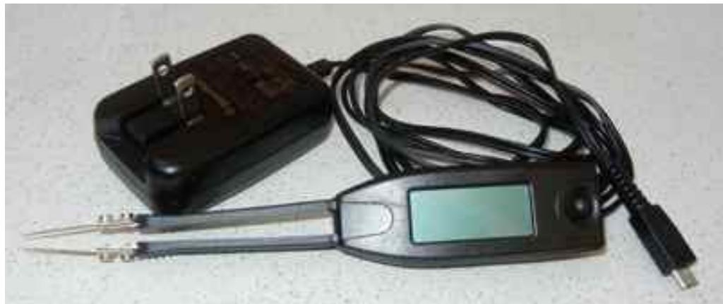
Smart Tweezers is a new patented design concept integrating a digital multimeter with a built-in gold-plated SMD probes and a display. This light weight device can be easily held by one hand. and is ideally suitable for component evaluation on a PCB or a production line and sorting of SMD components. Smart Tweezers dramatically reduces time necessary to troubleshoot or debug a PCB simplifying process of locating a faulty component.
